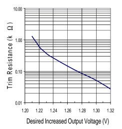
iHA48060A012V-001 Trim down curve for output voltage adjustment
